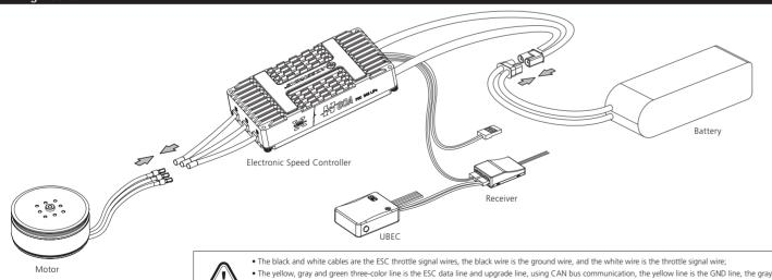
line is CH, and the green line is CL; • The CAN line is also a digital throttle line and can be used in parallel.
