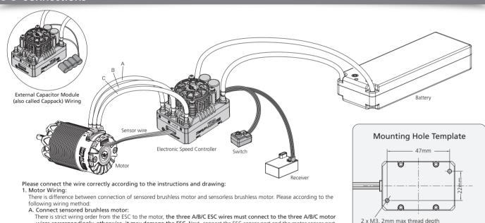
wires correspondingly, otherwise, it may damage the ESC. Next, connect the ESC sensor port and the motor sensor powith the stock 6-pin sensor cable. If you don't plug the sensor cable in, your ESC will still work in sensorless mode even
