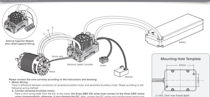
wires correspondingly, otherwise, it may damage the ESC. Next, connect the ESC sensor port and the motor sensor powith the stock 6-pin sensor cable. If you don't plug the sensor cable in, your ESC will still work in sensorless mode even
