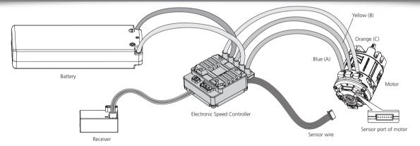
This is an extremely powerful brushless motor system. For your safety and the safety of those around you, we strongly recommend removing the pinion gear attached to the motor before performing calibration and programming functions with this system. It is also advisable to keep the wheels in the air when you turn on the ESC.
