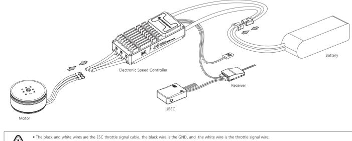
s the GND, the gray wire is CH, and the green wire is CL; The yellow, gray and green wires are the ESC data cable and upgrade cable, using CAN but • The CAN cable is also a digital throttle cable and can be used in parallel.
