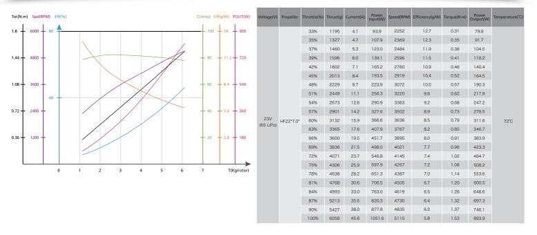
The above data are measured by Hobbywing Lab at the ambient temperature of 25 C and sea level by changing the throttle input adjustment. The motor temperature is measured by running the throttle at the rated point for 10 minutes, for reference only.
