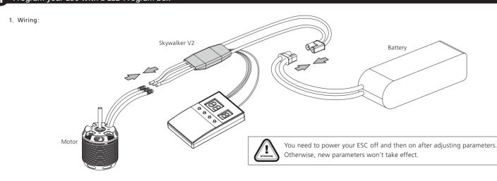
1) Plug the programming cable (on your ESC) into the programming port on the LED program box.
