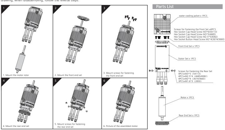
Note: The 2850 motor no screws to fix the front end cover. And both the front and rear covers of 2040 motor have no fixing screws.
